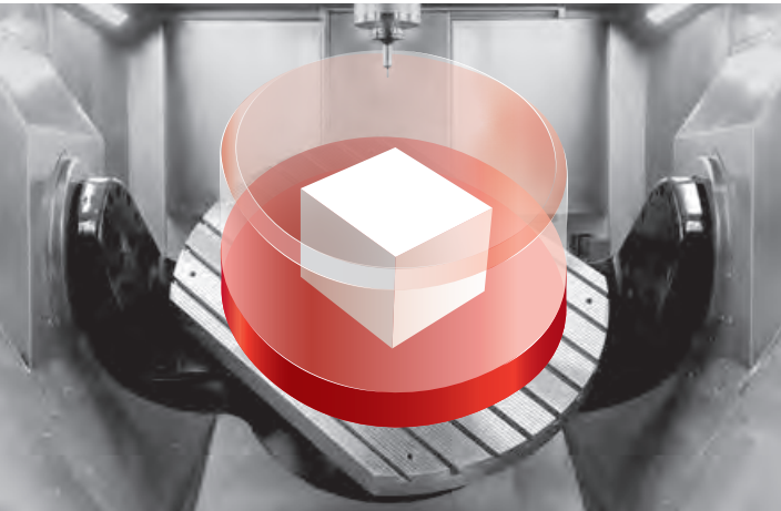
5-side positioning milling
